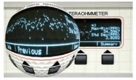
**Trending Measurements** – The ability to see measurement trends allows users an unparalleled look at the measurement cycle. Visually see the measurement affects when changing setup variables such as voltage polarities, integration times or capacitance values. Also see the measurement affects due to temperature, pressure or humidity changes. The 6520 allows you to see the complete or immediate measurement processes at your leisure, not ours. See what you have been missing!
